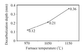
**Fig.2.** Main factor response diagram of decarburization depth and furnace temperature.
