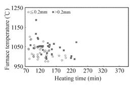
**Fig.5.** Scatter plot of furnace temperature and heating time for decarburization depth.
