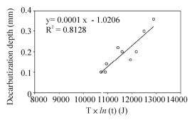
**Fig.4.** The regression analysis of decarburization depth and T\*ln(t).
