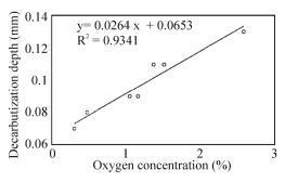
**Fig.6.** The regression analysis of decarburization depth and oxygen content.
