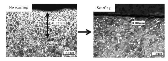
Fig.1. The change of decarburization depth in OM morphology for billet through the scarfing process.
